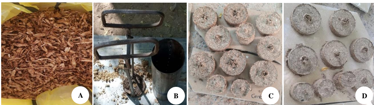
Figure 1. A. Bean chaffs; B. Manual piston briquetting machine, C. Untreated briquette samples, D. Treated briquette samples
