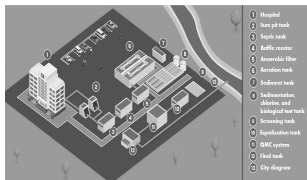
Figure 1. The schematic diagram of sampling sites of hospital WWTP of RSUDZA in Banda Aceh, Indonesia. The sum pit tank (No 2), aeration tank (No 6), and final tank (No. 12)
