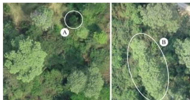
Figure 8. Significant factors responsible for the photogrammetry not being able to identify the trees: (A) suppressed or under a canopy and (B) continuous canopy in a dense growth of trees
