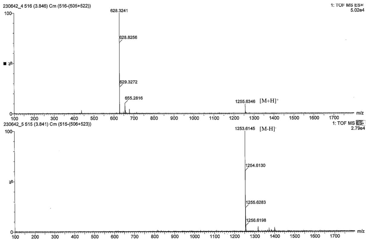
**Figure 4.** LCMS of actinomycin D. Method: cortecs column (2.1× 50 mm), 40%-100% CH<sub>3</sub>CN/H<sub>2</sub>O gradient for 5 minutes, flow 0.3 mL/min
