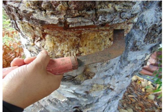
Figure 2. Specialized tapping knife developed for Gov. Generoso tappers
