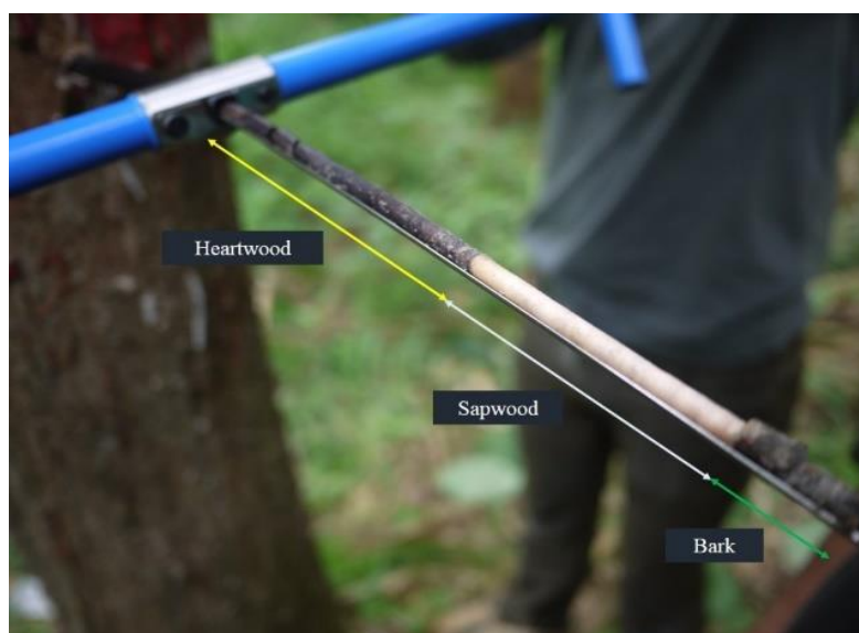
Figure 2. The collection of core sample using an increment borer
