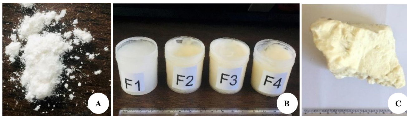
Figure 1. A. Extracted caffeine crystals; and B. Prepared four formulations with concentrations of 0, 0.5, and 1% caffeine; C. Incorporating chyuri butter
