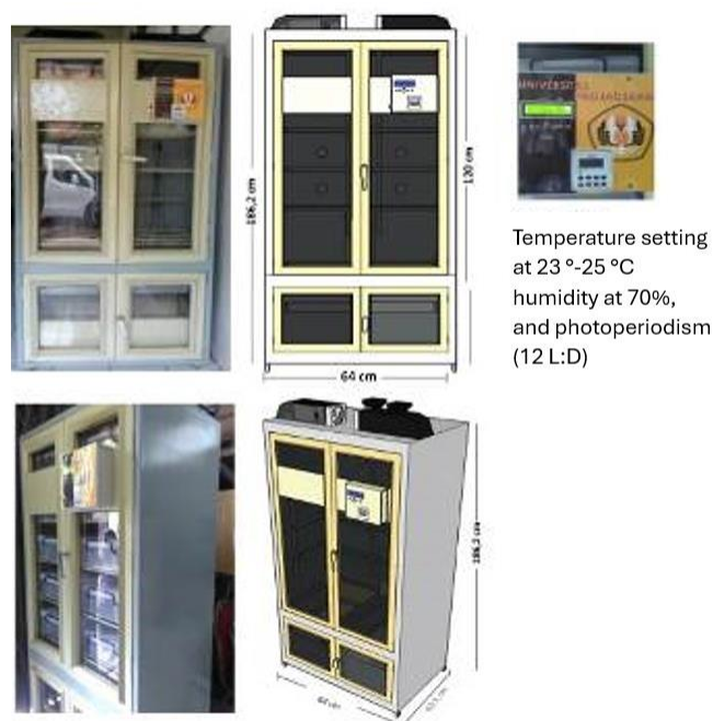
Figure 1. Insect-rearing cabinet with specified dimensions and controlled temperature, humidity, and lighting settings (Hermawan et al. 2017).
