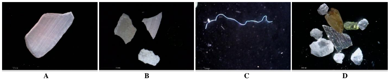
Figure 3. Examples of microplastics which were found on the coast of Manokwari, West Papua, Indonesia. A. Fragment; B. Foams; C. Fibers, D. Film
